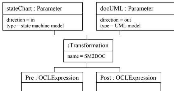
**Figure 5 – The SM2DOC model transformation specification**
