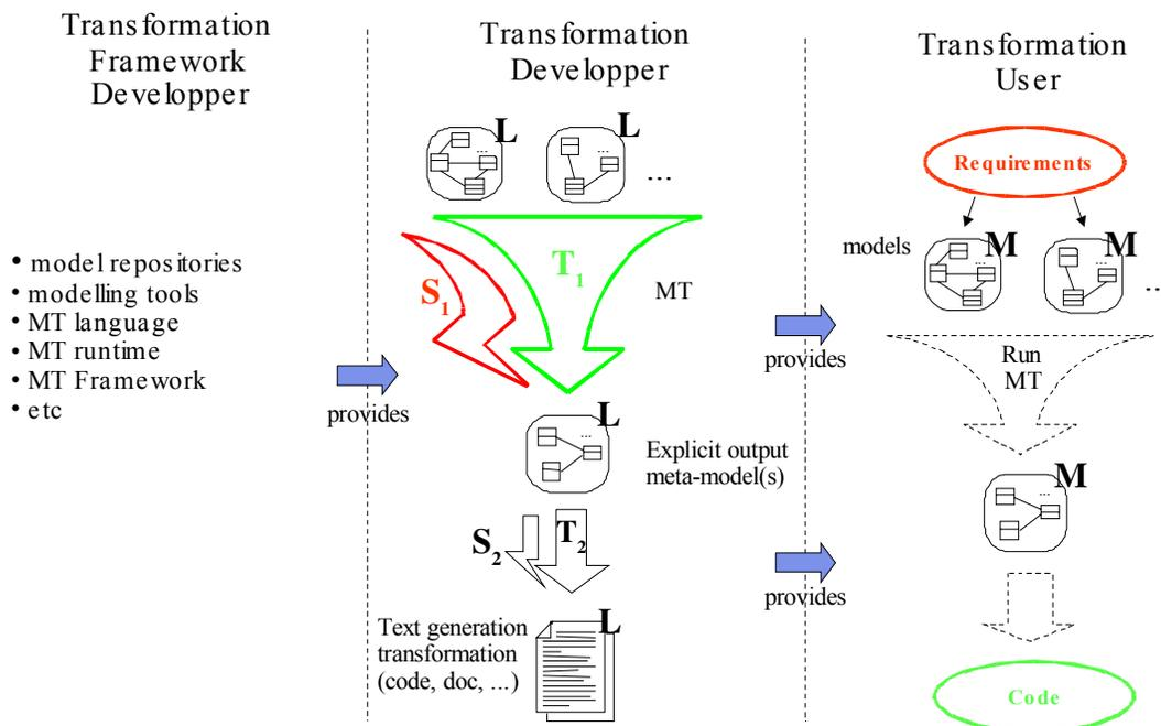
Figure 1 – Model-Driven Engineering Software Development Approach
